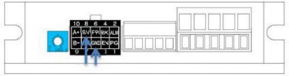
PWM speed regulation or analog input port
