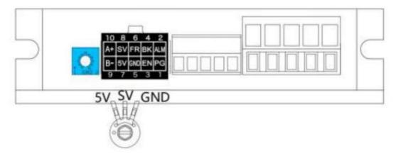
When the input voltage is about 0.2V, the motor speed is 5% of the maximum speed; When the input voltage is about 5V, the speed of the motor is at its maximum. The maximum speed value depends on the motor size and supply voltage.
