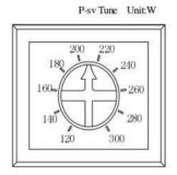
**Note:** To protect the motor, set the arrow number as the same as the motor nominated power. Whenever overload occurs the drive will turn out to be the protection mode.
