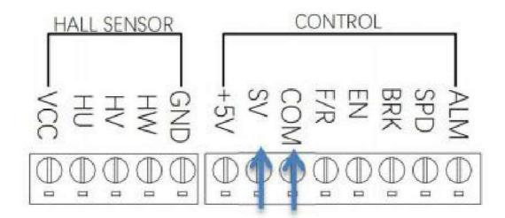
PWM speed regulation or analog input port
