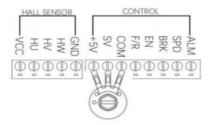
When the input voltage is about 0.2V, the motor speed is 5% of the maximum speed; When the input voltage is about 5V, the speed of the motor is at its maximum. The maximum speed value depends on the motor size and supply voltage.
